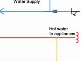
For CO2 heat-pump applications, size circulation pump for minimum flow rate required for pipe heat loss.
