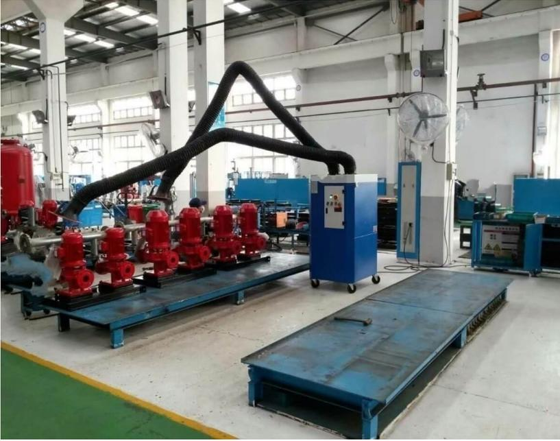
and air purification. HEPA filters can capture particles down to 0.3 microns in size, making them ideal for capturing and expelling welding fumes.
