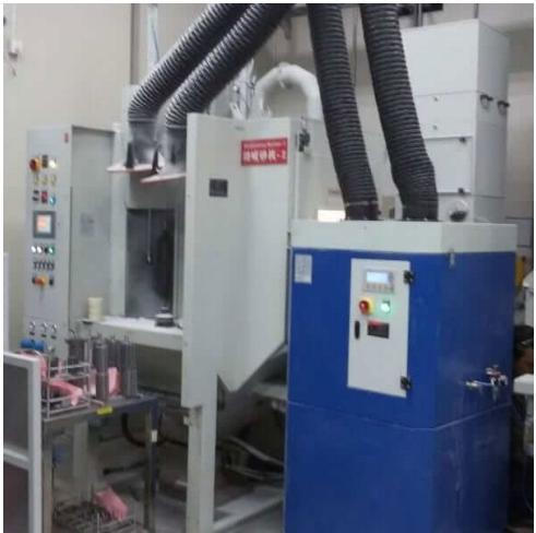
The SafeWork guidelines classify equipment that captures contaminants close to its point of generation as "local exhaust ventilation". The guidelines also state that the air from the system should not be recirculated in the work area but discharged away from workers.
